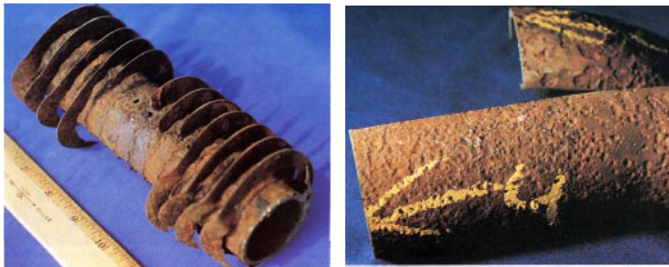
Figure 14. Examples of Tubes Corroded by Sulfuric Acid [7]
